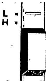
The Impact Control Selector, which is located to the right of the Pitch Selector, dictates to the printer how hard the characters on the daisywheel will strike the page. You have a choice of two settings: L (light) and H (heavy).
